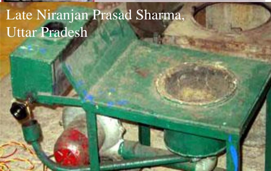
Pre-heating of kerosene improved fuel efficiency 35-60 per cent
