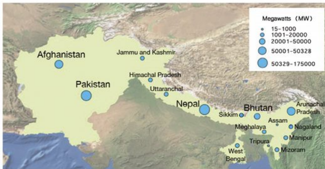
The total estimated hydropower potential in the Hindu Kush Himalaya (HKH) – with China's HKH region included – is 500,000 MW © ICMOD.
