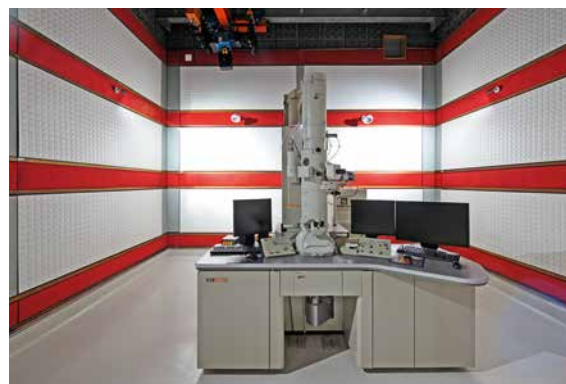
Above: High resolution transmission electron microscope at CHRTEM, Nelson Mandela Metropolitan University.
