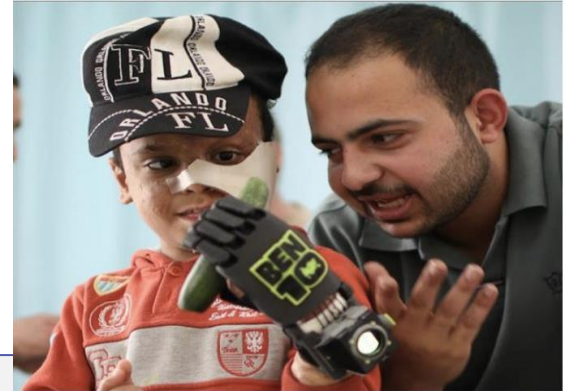
The hand was 3D-printed in carbon fiber-reinforced co-polyester material for under $75 on a $1700 Ultimaker 3D printer by Asem Hasna, a Syrian refugee on the ROW team who learned 3D printing in three weeks. (image via 3ders.org)
