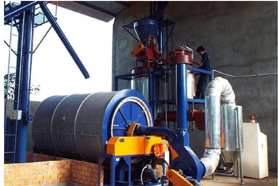
Pyrolysis machine designed by Okozentrum, carbonizing coffee husks and generating energy in Vietnam
