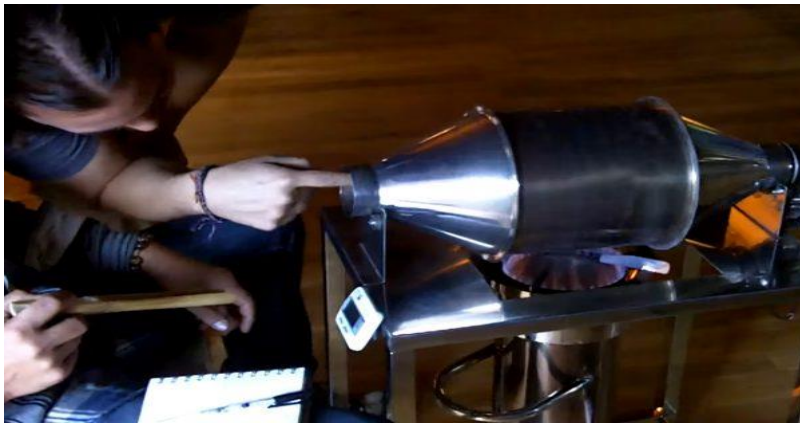
Running a micro gasifier with coffee pulp to roast coffee beans and make biochar in Laos.
