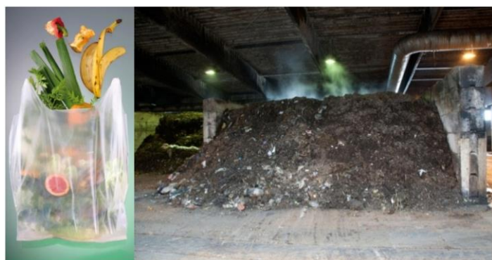
Figure 5. Biobased and certified biodegradable organic waste bags are applied to collect organic waste from e.g. households and are finally composted in a professional composting facility all together with the organic content.
