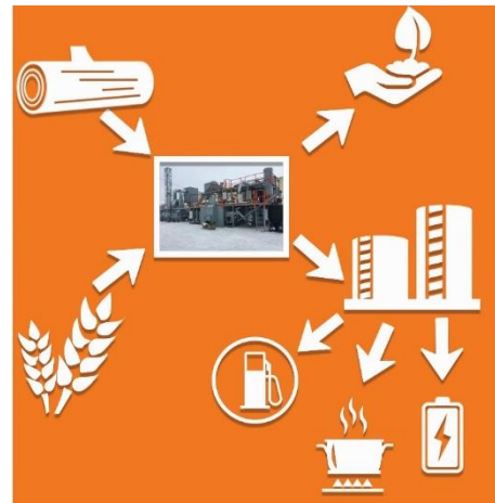
Figure 3. Inputs and outputs of ablative pyrolysis. Biomass inputs are converted into biochar or bio-oil that can be sent to a refinery to produce fuels. Pyrolysis reactor: Copyright 2020 Biogas Inc
