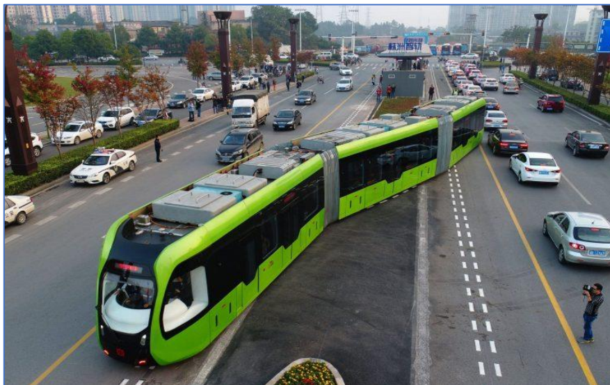
Figure 1: The Trackless Tram System developed by CRRC and demonstrated in Zhuzhou, China.
