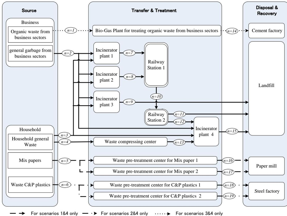
Figure 8: MSW processing flow scenario analysis in Kawasaki
